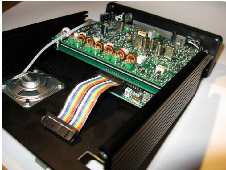
Ready to slide in the analog modules from the back of the case. First mount the speaker and erectable foot.
