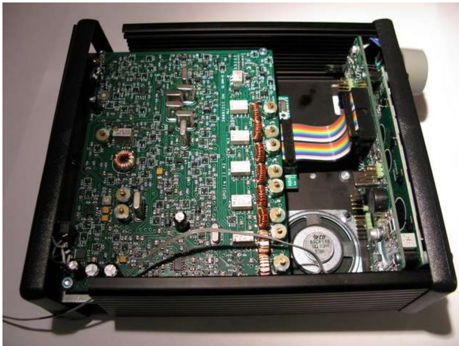
The back of the rig is to the left and the front to the right. Slide in the top panel before putting in the top countersunk screws.
