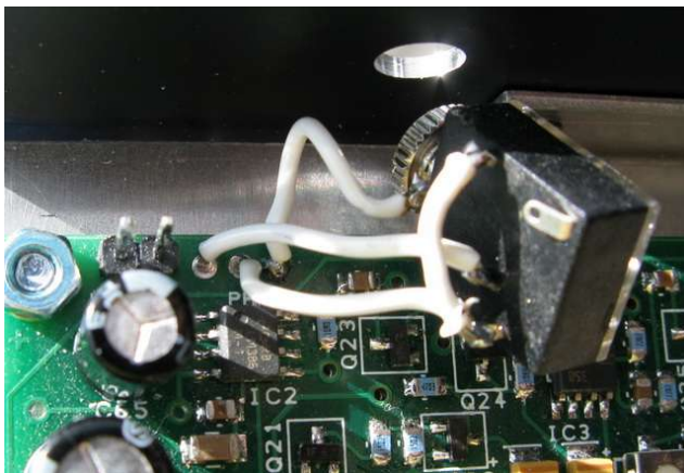
External speaker connector. The jumper is used for 3 pole 3.5 mm connector
