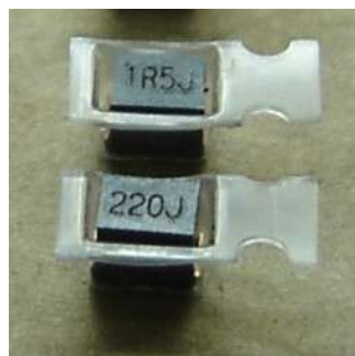
Inductors: The one on top is 1.5uH, Bottom 22uH.
