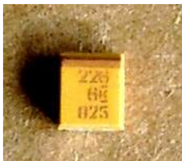
This is a Tantalum capacitor. "226" means that it is a 22uF.
