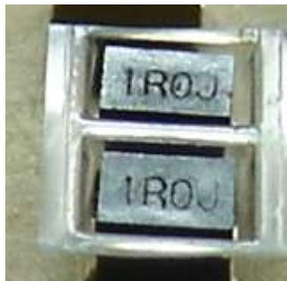
These are two 1uH Inductors. Don't be confused by the "R" to believe it is a resistor.
